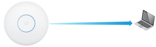
SU-MIMO: A Wave 1 AP communicates with one client at a time.
